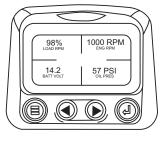
2. The main menu will pop up on the display. Use the "Arrow Buttons" to scroll through the menu until the "Engine Configuration" menu item has been highlighted.
